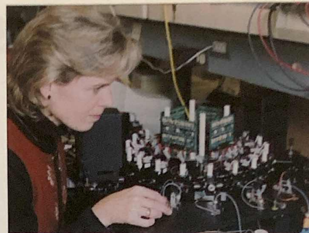
Meldrum observes the Acapella-5K as it rotates through samples. This system has automated and increased the speed of sample handling for DNA sequencing by 10 to 100 times. Photo: Kathy Sauber/UW Photography
