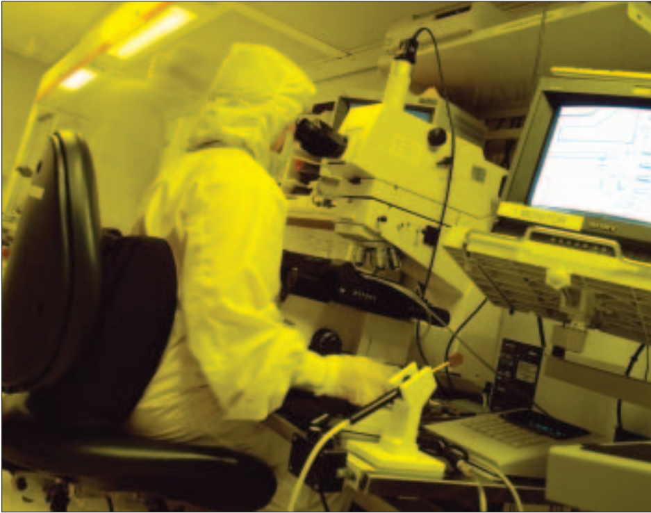
In a dust free environment, materials like chromophores are integrated into wafer chips. Photo: Agilent Technologies
